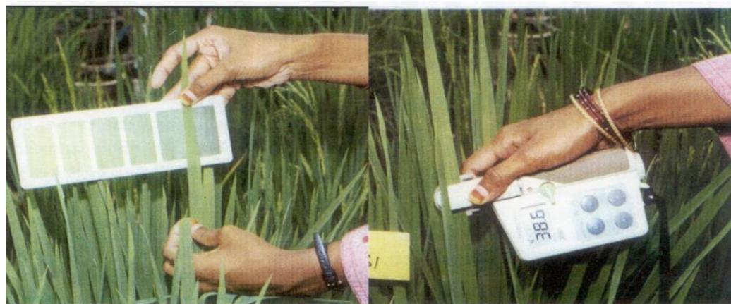
Leaf color chart (left) is found to be an inexpensive alternative to SPAD chlorophyll meter (right) for effective N top dressing
